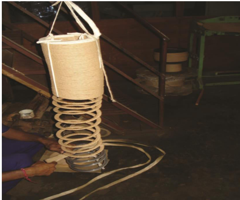
Fig. 1: Winding insulating process...
