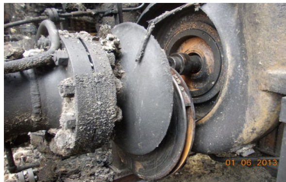
Detached Impeller from the shaft
